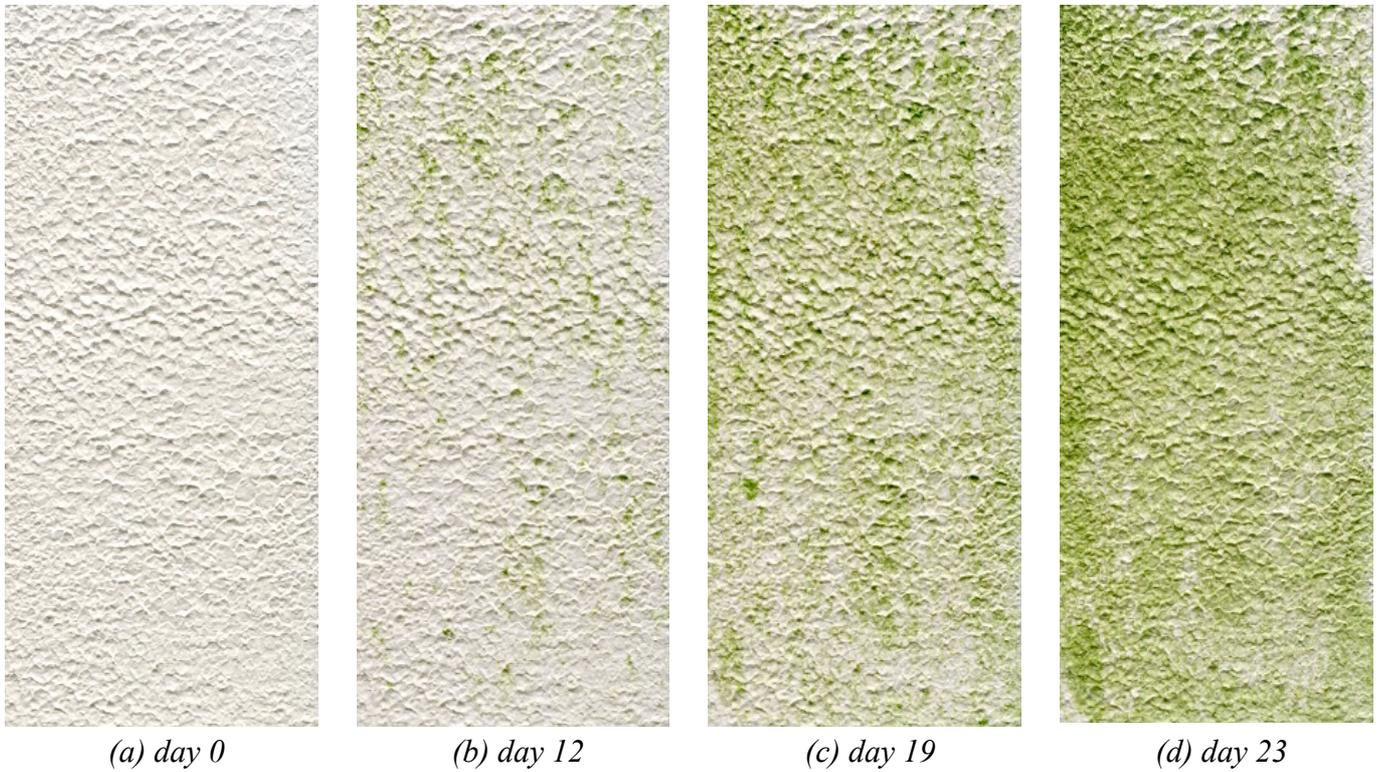
*Figure 1: Examples of image of a mortar colonized by algae at different time.*
